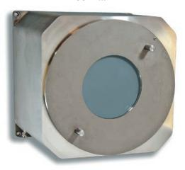
CCAIF and CCAIF...H series junction boxes in stainless steel have a **screw cover** with or without round window. They are used either as junction boxes with/without terminals and the body and cover can be drilled and threaded according to customers' specification. In accordance with rules, Cortem only can perform the drilling.
