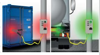
Therefore, with a capacitive earthing system, if an operator connects the pliers to a simple metal element it recognises that it is not connected to a tanker truck and does not allow the loading/unloading of the liquid.
