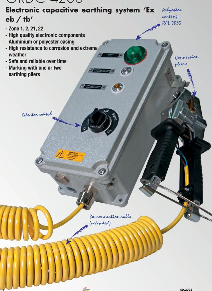
The GRDC-4200 is a capacitive-type electronic earthing system that ensures earthing of tankers, rail tankers and IBCs (intermediate bulk containers) when transporting flammable liquids such as fuels, chemicals, powders and granulates.
