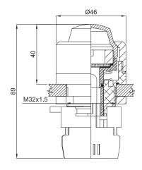
Illuminated push-button with standard 10A 600V 1NO+1NC contacts. (lamps on request) Illuminated button comes in choice of five colours.
