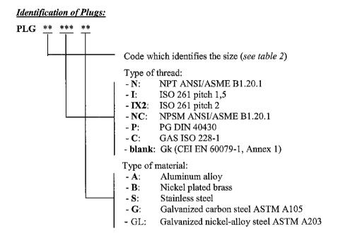
Sizes and threads of special Adaptors and Plugs are listed on the following Table 2.
