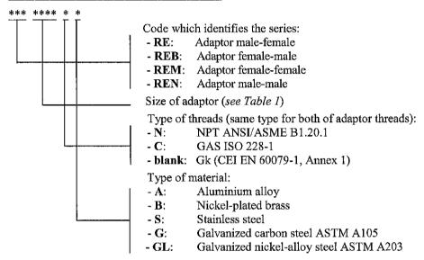
Standard sizes and threads of Adaptors series RE.., REB.., REM.. and REN.. are listed on the following Table 1:
