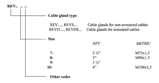
Range of non-armoured cable passage of the cable glands "ELFIT" type REV.., REVS size 7 ÷ 10
