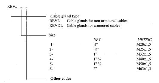
Range of non-armoured cable passage of the cable glands "ELFIT" type REVL... size from 1 to 6.
