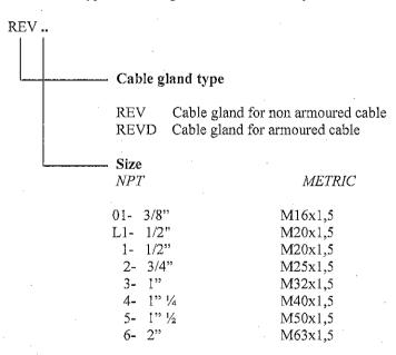
Other suffix can be added on the code for particular configurations: REVN... - REFV... (\*)
