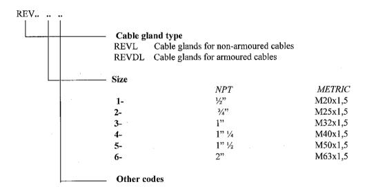
Range of non-armoured cable passage of the cable glands "CORTEM" type REVL... size from 1 to 6.
