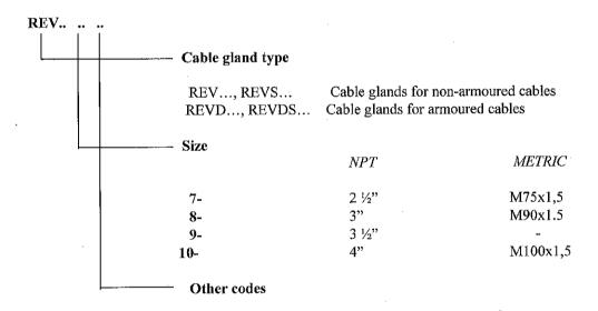
Range of non-armoured cable passage of the cable glands "CORTEM" type REV.., REVS size  $7 \div 10$
