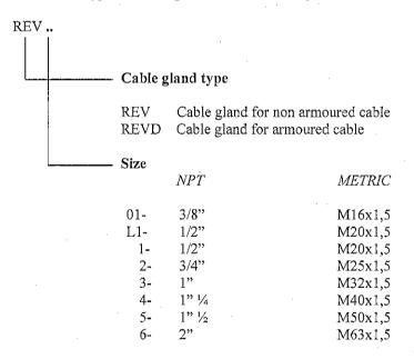
Other suffix can be added on the code for particular configurations: REVN... – REFV... (\*)
