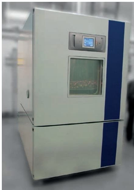
Fig. 18 Climatic cell in the Cortem Group laboratory where the product heat resistance is tested
