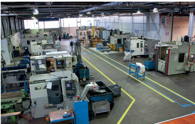
Fig. 17 Part of the workshop fitted with horizontal and vertical processing stations, CNC lathes, transferring machine and equipment.
