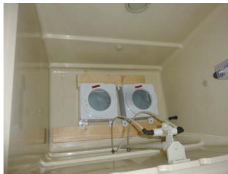
Fig. 20 Enclosures tested in salt mist
