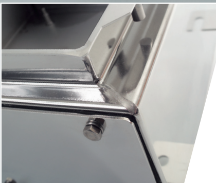
Detail of TIG welding of walls
