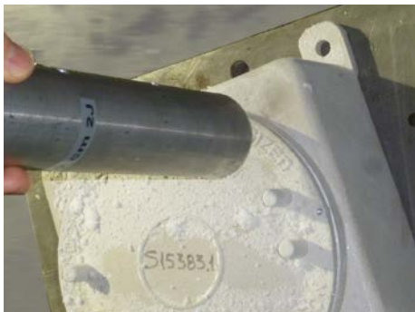
Fig. 19 Impact test at 7J on a GUB series box after a cycle in a climatic cell at -65°C
