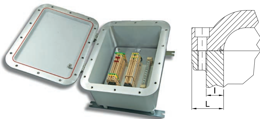
Fig. 12 EJB series 'Ex d' enclosure where you can see the rolling joint, where the distance "l" is the length of the flat section between the inside of the enclosure and the hole, while the distance "L" is the length of the rolling joint, that must be in compliance with the provisions of the IEC/EN 60079-1 standard, per type of execution (IIB or IIC).
