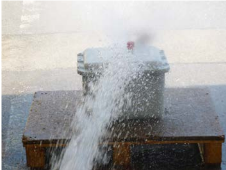
Fig. 21 IP X6 protection degree test
