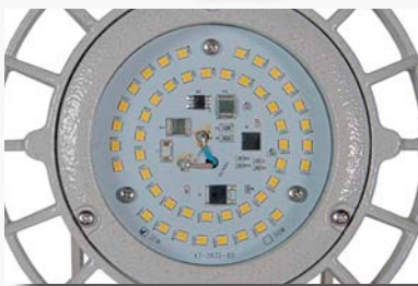
LED resin-bonded electronic board
