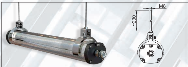
Ceiling mount with 250 mm rod
