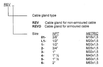
Other suffix can be added on the code for particular configurations: REVN... - REFV... (\*)
