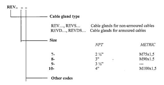
Range of non-armoured cable passage of the cable glands "CORTEM" type REV., REVS size 7 ÷ 10
