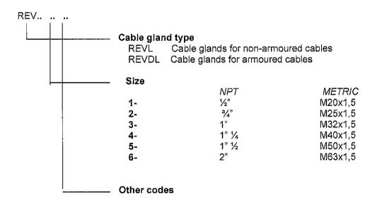
Range of non-armoured cable passage of the cable glands "CORTEM" type REVL... size from 1 to 6.
