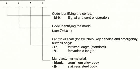
Other suffix can be added on the code for particular configuration, type of external handles or internal lever.
