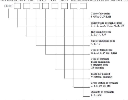
When the code starts by "SF", the box is supplied complete with bracket for wall mounting (ex. SFC-26.1). When the code starts by "SSC", the box is supplied complete with bracket for ceiling mounting (ex. SSC-26.1). Other suffix can be added on the code for particular configuration.
